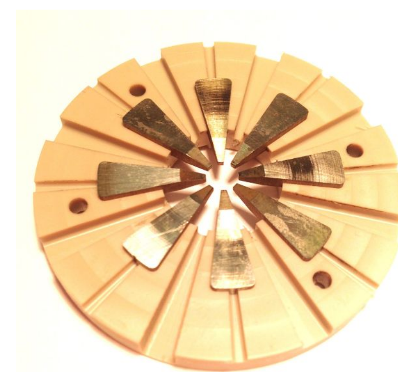
Figure 2: Barium ion Paul trap used in the University of Washington ion trapping lab. This trap uses eight planar electrodes and two axial electrodes to make 2D ion crystals.
